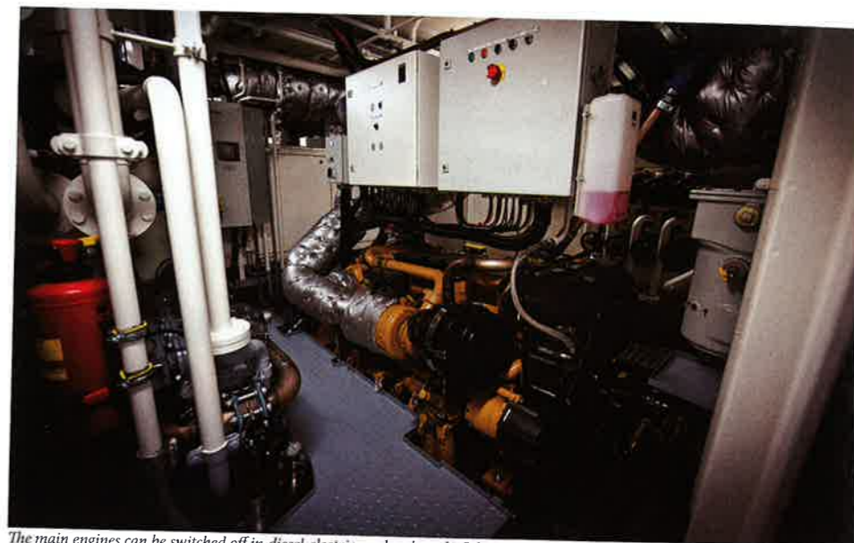
The main engines can be switched off in diesel-electric mode, photo by Edu Calicher
