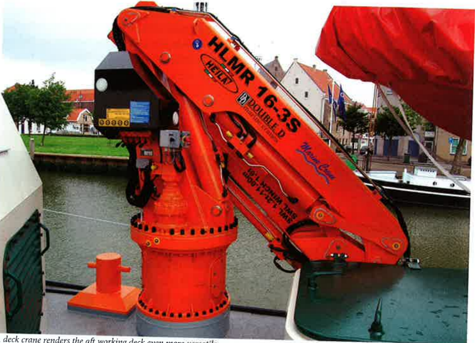
A deck crane renders the aft working deck even more versatile
