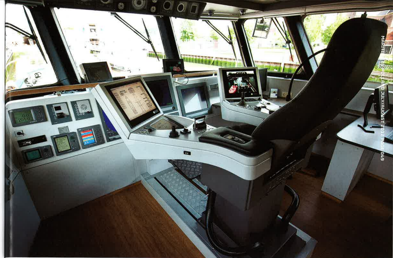
Regularly used navigation functions are integrated into the helm seat armrests, photo by Edu Calicher
