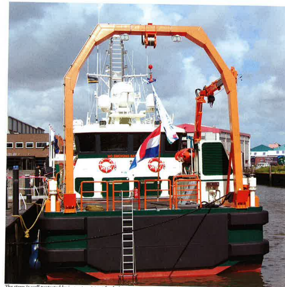
The stern is well protected by impact-resistant fendering
